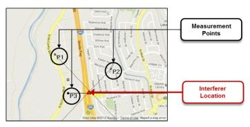
Fig 16. Triangulating the Interferer
