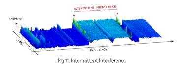
VIAVI RF Test analyzers perform spectrogram measurement that can be executed in an unattended manner for several days, continuously recording the results and having the ability to perform post-analysis of the results. This provides useful information to identify and locate the interference signal.
