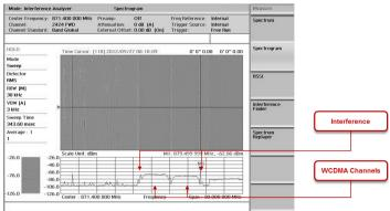
Fig 12. Detecting Intermittent Interference Signals
