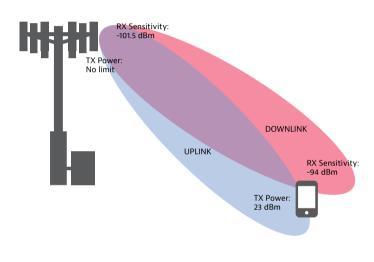
Fig 2. LTE-TDD (10 MHz) Transmission and Sensitivity Requirements
