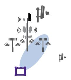
Fig 15. Interference Location with Directional Antenna
