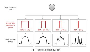
For this reason, one must set the adequate RBW in order to have enough resolution and measurement time to detect interference signals. In general, the maximum value of RBW to properly identify a signal is 25 percent of the signal's bandwidth. For example, to properly detect a GSM signal (a narrow-band, 200 KHz signal) the RBW should be lower than 50 KHz.
