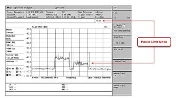
Fig 10. Spectrum Clearance Mask
