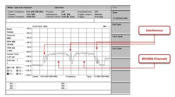
Fig 13. WCMDA Channels with Interference
