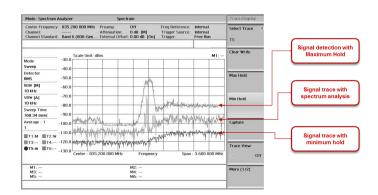
This methodology is perhaps the first measurement taken on spectrum with suspected interference, and the basis to proceed with an interference analysis such as the signal occurrence or periodicity through a spectrogram testing.
