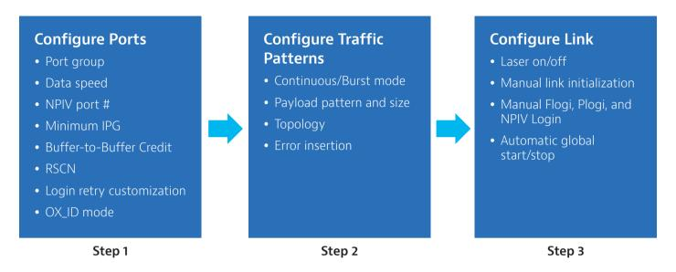
Configuring Xgig Load Tester with a simple three-step process
