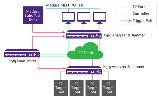
Example setup with the Xgig Load Tester and VIAVI Medusa Labs™ Tools for testing Fibre Channel fabric performance.
