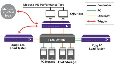
Figure 1: Example setup with the Xgig Load Tester and Medusa Lab Tools for testing FCoE switch performance.
