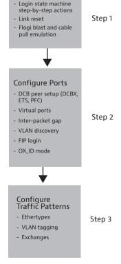
Figure 2: Configure Xgig Load Tester with a simple three-step process
