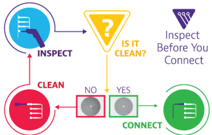
Figure 2: Inspect Before You Connect
