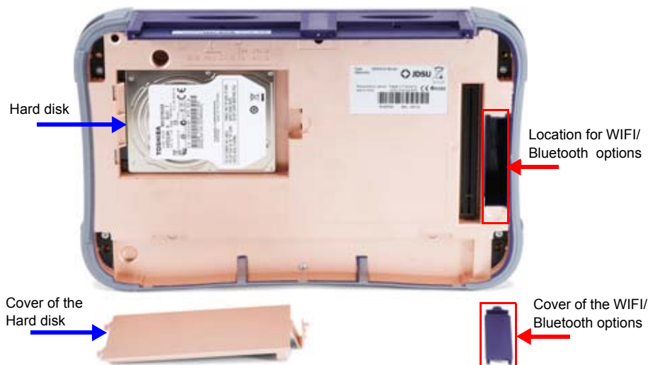
Fig. 88 Location for the hard disk and WIFI/Bluetooth options
