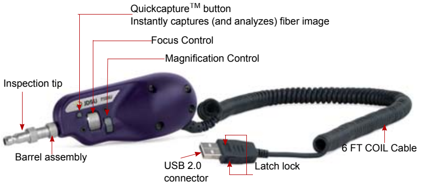
Fig. 14 P5000i Probe components
