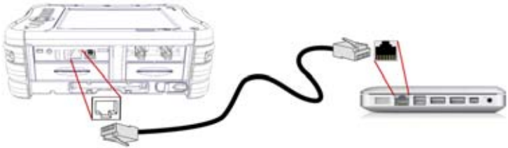
Fig. 34 Connection 6000A V2 Platform and PC
