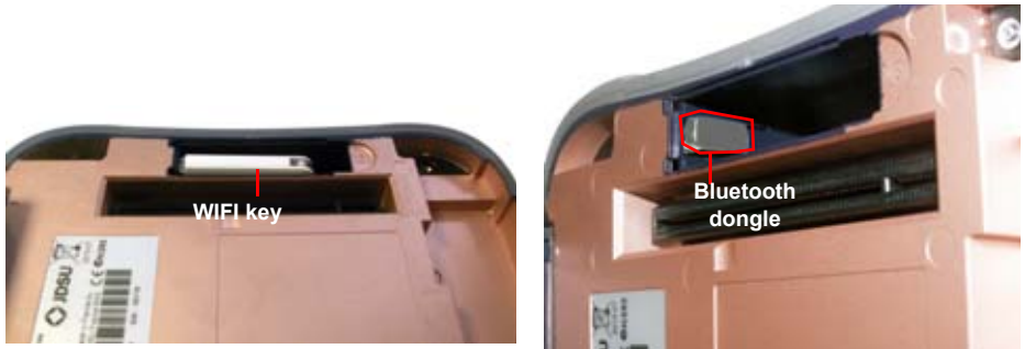
Fig. 89 WiFi / Bluetooth option installation
