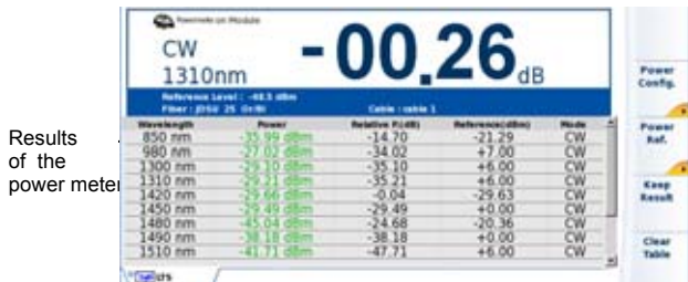
Fig. 12 Results and commands of the power meter
