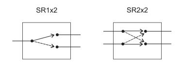
Solid lines represent the unpowered (0 V DC) state of the switch.
