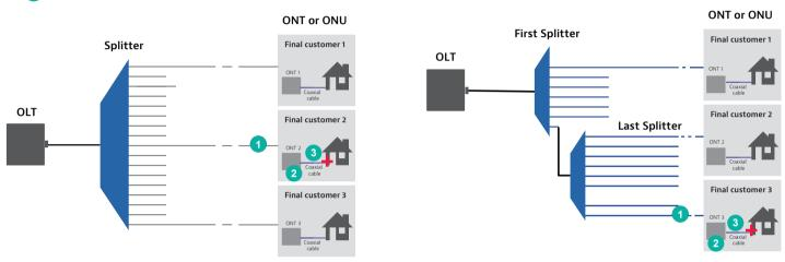
Figure 4. PON Case 1—Possible Faults When Only One Subscriber is Affected
