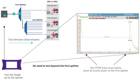
Figure 12. OTDR is Shot Downstream and Trace should Display the Traffic Down to the First Splitter
