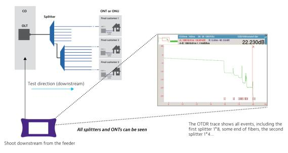
Figure 13. OTDR is Shot Downstream and Trace Displays Many Events that are Difficult to Identify without Exact Network Topology (and corresponding distances)
