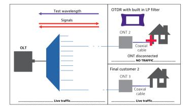
Figure 8. OTDR Insertion for In-service Monitoring
