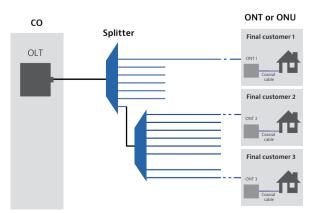
Figure 2. Simple PON Network Topology
