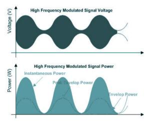
The upper graph of the above diagram shows the voltage envelope of a high frequency modulated signal. The lower graph shows the instantaneous power envelope of this signal, and the envelope power.
