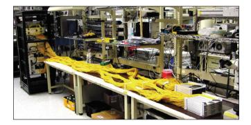
Figure 6: A JDSU OCETplus system is prepared for baseline referencing. The 5 m pigtails from the DUT switches are spliced together. Splices are managed on trays with strain relief holders.
