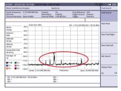
Interference observed at ground level
