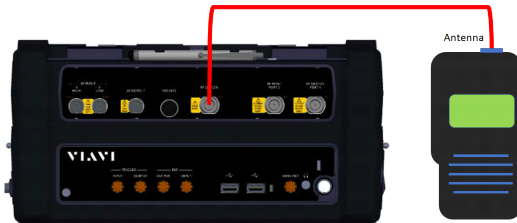
Figure 3-1 DMR Transceiver Test Setup Diagram
