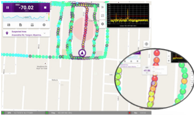
InterferenceAdvisor guides the engineer to the most probable interference source location
