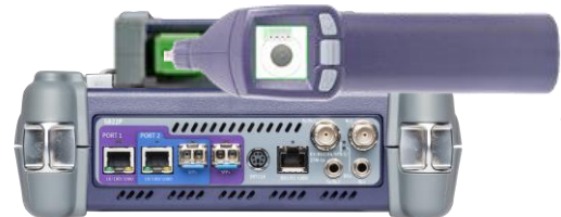
Figure 3: OTDR Port Inspection
