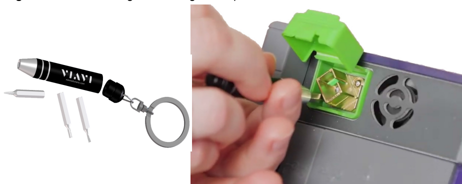
Figure 4 Removing and refitting an adapter
