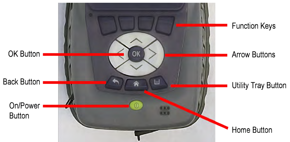
Figure 1-2 CX100 Controls and Buttons
