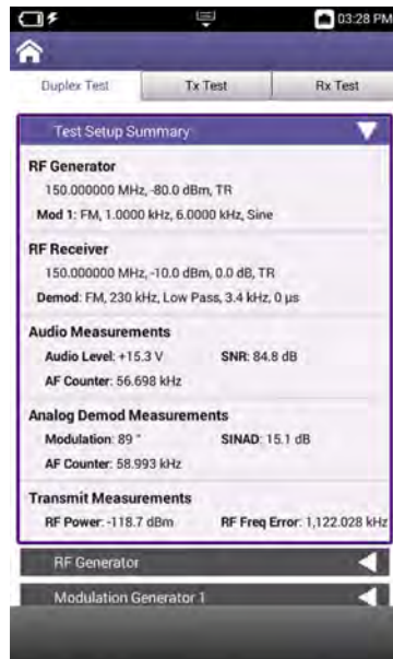
Figure 5-2 RF Test Setup Summary Panel
