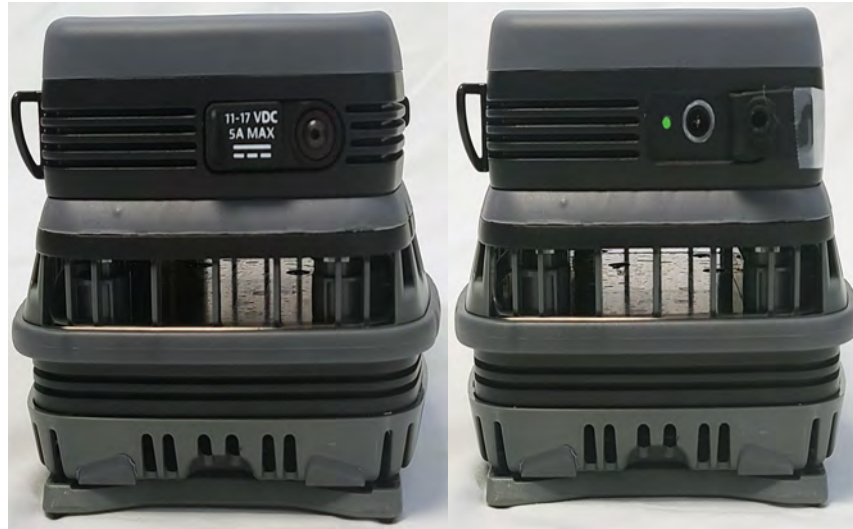
Figure 1-5 DC Input Connector Location
