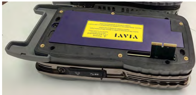
Figure B-3 Base Unit - RF Module Removed
