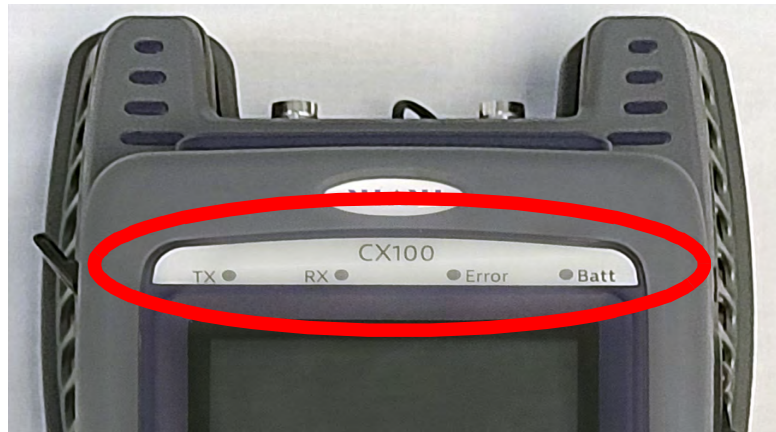
Figure 1-6 CX100 Front Panel LEDs
