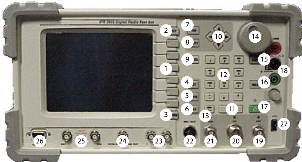
Fig. 3-2 3920/3920B Front Panel Connectors
