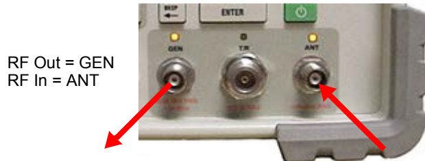
Fig. 3-29 GEN/ANT Two Port Duplex Test Setup
