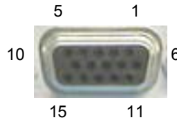
Fig. 2-9 VGA Monitor Output Pin Locations
