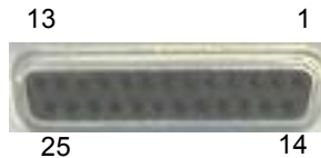
Fig. 2-8 Parallel Connector Pin Locations
