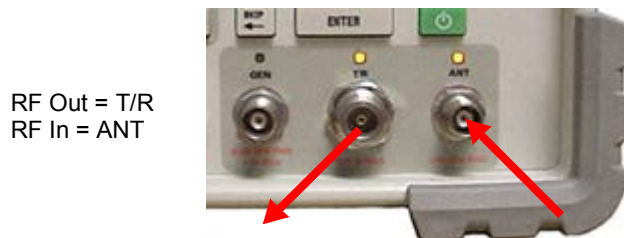
Fig. 3-31 TR/ANT Two Port Duplex Test Setup
