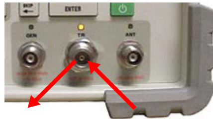
Fig. 3-28 One Port Duplex Test Setup
