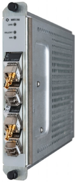
WaveReady WRT-780/781: 4-port Flexible C/DWDM 4.25 Gbps Transponder
