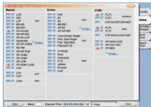
Figure 3: ONT-503/506/512 alarm overview
