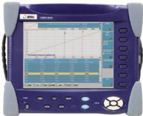
T-BERD® 8000 Modular Test Platform OTDR, IL, ORL, PMD, CD, AP, CWDM OTDR, Link Characterization 1 , Inspection
