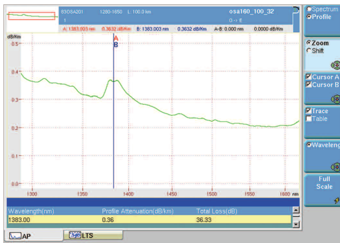
Figure 7. Attenuation Profile measurement with the T-BERD®/MTS-8000 and a full band broadband source (1260 to 1640 nm)
