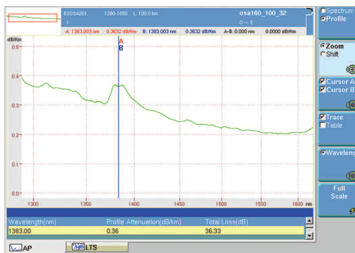
Figure 6. OTDR measurement at 1383 nm with the JDSU VLR module
