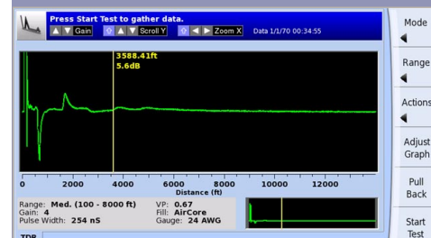
Example of a copper trace (TDR)
