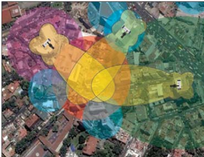
Fig 11 – Interference location through triangulation
