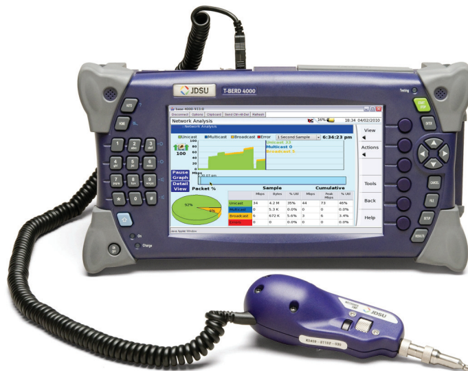
Figure 14: JDSU T-BERD/MTS-4000 platform with the ESAM
