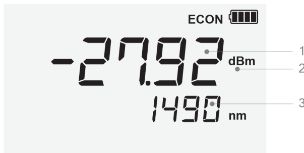
Fig. 11 Absolute power measurement
