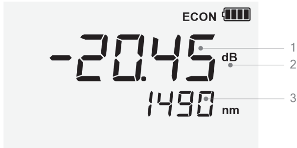
Fig. 12 Relative power measurement
