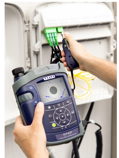
SmartClass Fiber system with integrated power meter and patch-cord microscope
