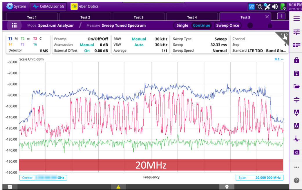
CellAdvisor 5G – Spectrum Analysis TDD Carrier with Intermittent Interference
