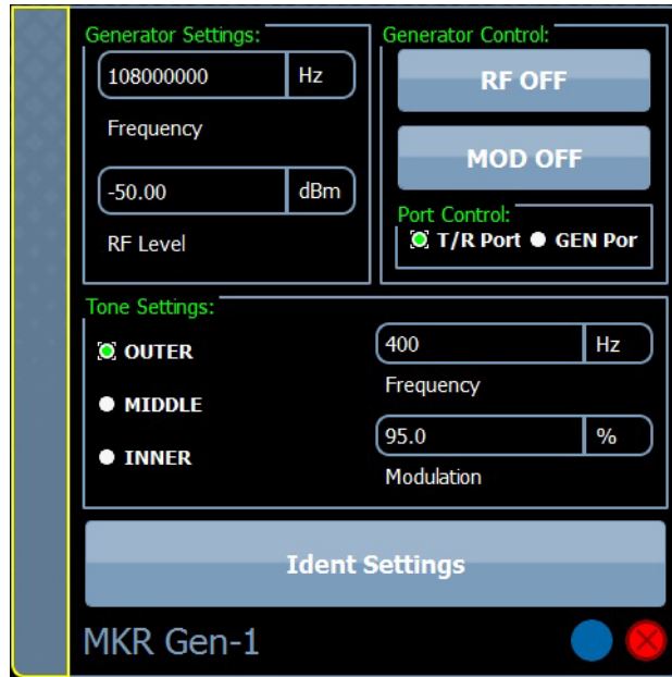
Fig. 2-21 MKR generator GUI
