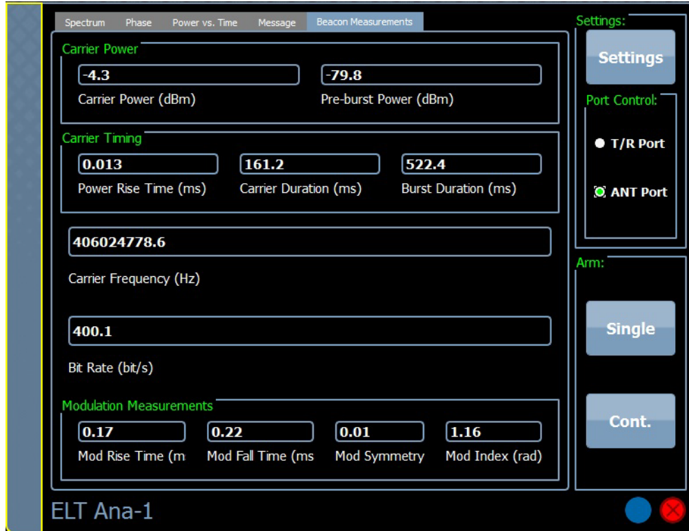
Fig. 2-55 Beacon Measurements Screen
